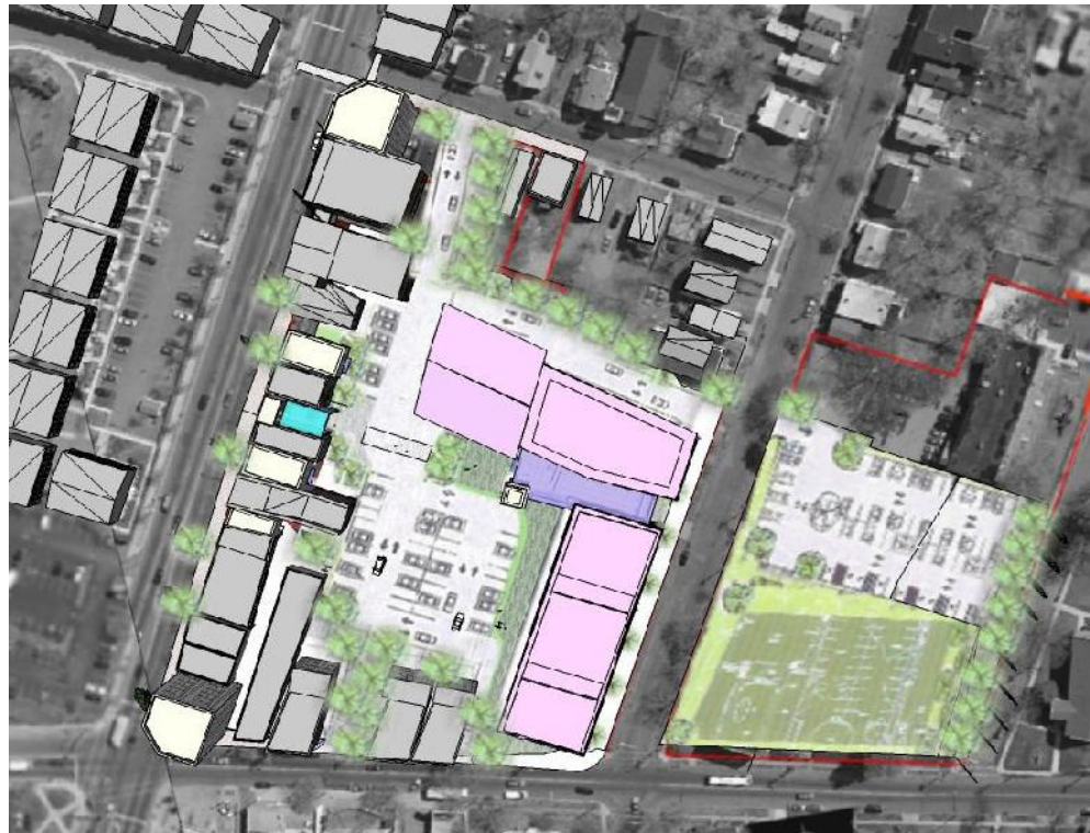
Figure 5.5: Aerial view– Elm Street looking east. Note courtyard entry to school’s public amenities from Bloomfield Ave. Higher density uses are near Bloomfield Avenue, with school/retail shared parking. Sports field and secondary parking south of Washington Street, in deference to neighborhood’s residential character (Scenario 1).
